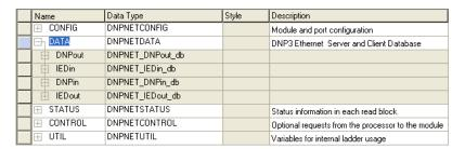
Notice these UDTs are the data types used to declare the DNPNET.DATA controller tag arrays.
