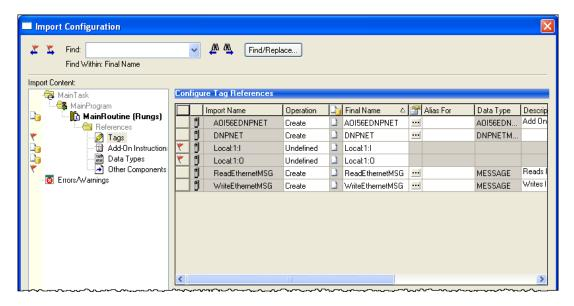
10 Associate the I/O connection variables to the correct module in the corresponding slot number. The default values are Local:1:I and Local:1:O and must be edited if the card is placed in a slot location other than slot 1 (Local:1:x means the card is located in slot 1). Since the second card is placed in slot 2, edit the FINAL NAME to Local:2:I and Local:2:O.
