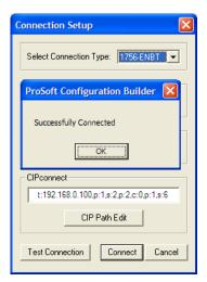
8 Click **OK** to close the Test Connection pop-up and then click **CONNECT** to close the *Connection Set* up dialog box. The Diagnostics menu is now connected through CIPconnect.
