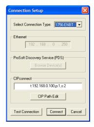
5 If the Test Connection is successful, click CONNECT to display the Diagnostics menu in the Diagnostics Window.
