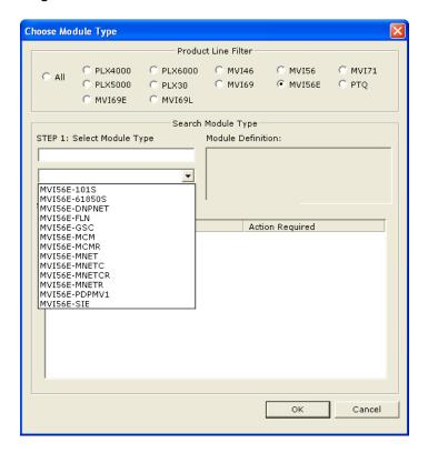
3 In the *Product Line Filter* area of the dialog box, select **MVI56E**. In the *Select Module Type* dropdown list, select **MVI56E-DNPNET**, and then click **OK** to save your settings and return to the *ProSoft Configuration Builder* window.
