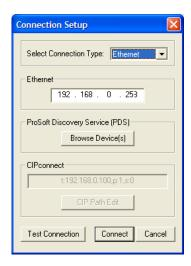
You can also use CIPconnect® to connect to the module through a 1756-ENBT card by choosing 1756-ENBT in the **Select Connection Type** list. Refer to Using CIPconnect® to Connect to the Module (page 52) for information on how to construct a CIP path.
