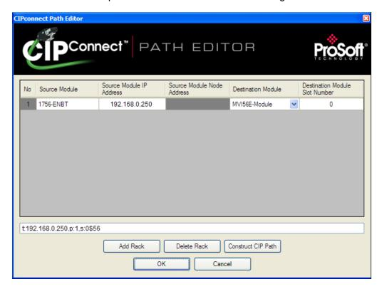
The *CIPconnect Path Editor* allows you to define the path between the PC and the MVI56E-DNPNET module. The first connection from the PC is always a 1756-ENBT (Ethernet/IP) module.
