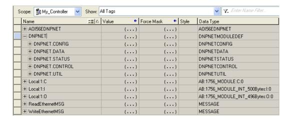
Some UDTs hold process or status data (*Module Data Objects*). This data can be monitored and manipulated by the application-specific ladder logic program. Other UDTs are used to store and organize the parameters needed for special functions and control features (*Special Data Objects*). These data types will be discussed in more detail in succeeding topics.
