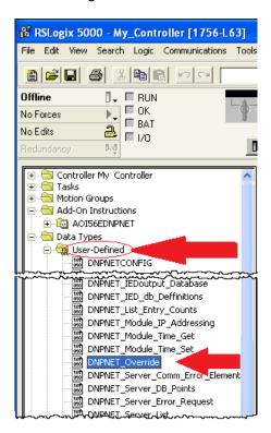
Double click the *DNPNET\_Override* UDT. A window opens and displays the Members of this UDT. Notice the Members have similar names to the DNPNET tags to be edited. In the DataType column, the size of the specific tag array is determined by the value within the [].
