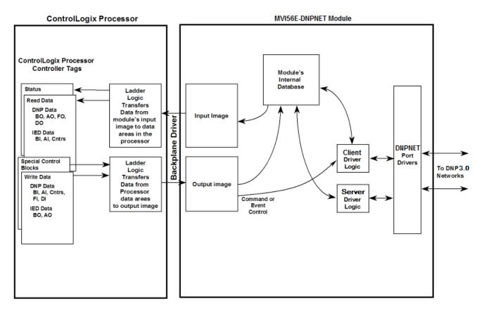
All data transferred between the module and the processor over the backplane is through the input and output images. Ladder logic is needed in the ControlLogix processor to interface the input and output image data with data defined in the Controller Tags. All data used by the module is stored in its internal databases. These databases are defined as a virtual DNPNET data tables with addresses from 0 to the maximum number of points for each data type.
