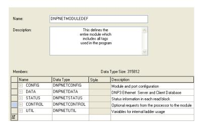
Click the [+] signs to expand the UDT structures and view lower-level UDTs. For example, when DATA is expanded, it contains four UDTs: DNPout, IEDin, DNPin, and IEDout. They can further be expanded with the [+] sign.
